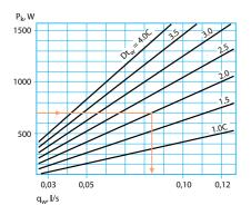
Correction for water flow, on basis of the diagram "Correction of cooling effect for water flow other than 0.05 l/s" is obtained K = Pk 0.083/Pk 0.05 = 1.05. The actual effect is therefore 5 % higher than the result given by the diagram, due to the higher water flow.
