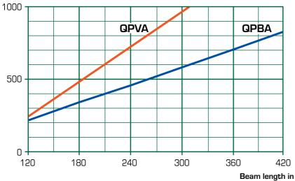
The diagram shows the approximate cooling effect, Ptot in W with water flow, qv = 0.05 l/s difference between room air temperature and average water temperature = 8 °C and max sound pressure level LA10 = 30 dB(A). 1)
