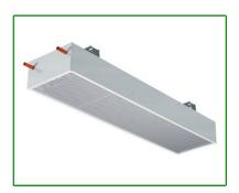
The Flexicool® QPVA and QPBA passive chilled beams provide for the cooling in a room. QPVA (width 570 mm ) and QPBA (width 430 mm ) are broad passive chilled beams. The passive chilled beams are either ceiling installed, in which case they lie flush with the suspended ceiling, or free space installed without ceiling.
