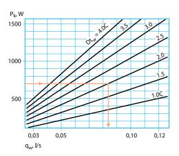
Note! The diagram is based on tests performed according to the method V (future Nordtest), which gives a very small temperature difference between the air entering the beam and the average temperature at 1.1 m above fl oor surface. In actual conditions with relatively concentrated heat sources, the temperature difference can be 1-2
